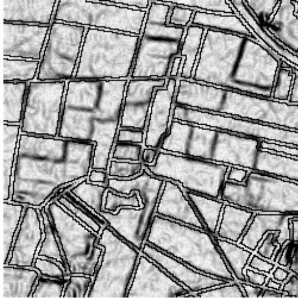
Fig. 5. Map aligned with edge-filtered SAR image using an affine transformation (the outline of the map boundaries is displayed rather than the boundaries themselves).
