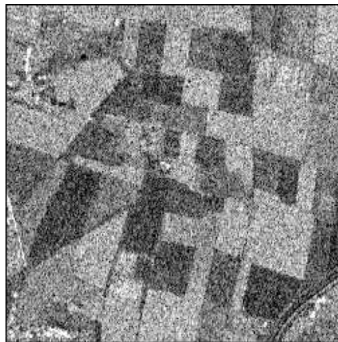
Figure 2: Synthetic aperture radar (SAR) image of area near Thetford forest, England. Values range from 0, displayed as black, to 255, displayed as white.
